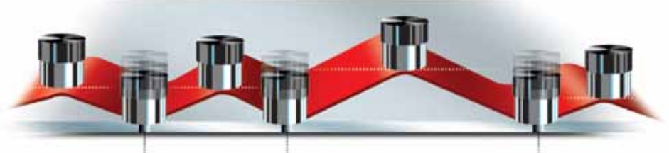
Smart Stroke® automatically selects the optimum hover height for each table move.
