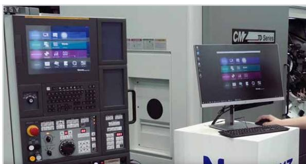
Once you are connected you will see the machine screen. However, in order to change modes and other things the machine panel, CMZ has developed a CMZ Virtual Operator Panel. For safety reasons start program and machine movements are removed from this option.
