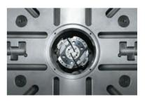
Integral Rotary Encoder The C-axis is equipped with a rotary encoder, enabling superb positioning accuracy and repeatability for precision machining.
