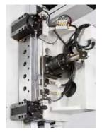
Once the rail is in place, hydraulics clamp the guide-ways and pin vertical position. This ensures perfect perpendicularity and rigidity with every positioning.
