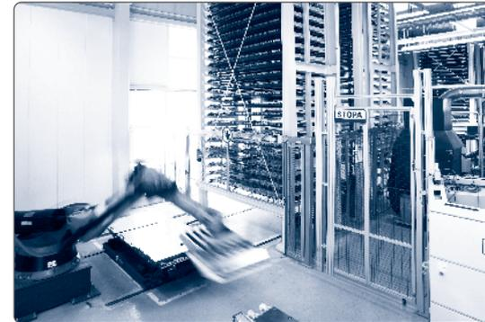
Connection of production machine with robotic loader
