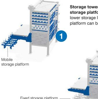
Storage tower, lifting beam and mobile storage platform: To permit access to the lower storage locations too, the mobile storage platform can be moved.
