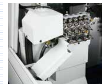
Work catcher Conveying the workpiece discharged from back spindle through the chute
