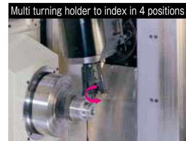
The tool can be indexed at fixed positions in 90 deg steps (4 positions) and tools can be used efficiently.
