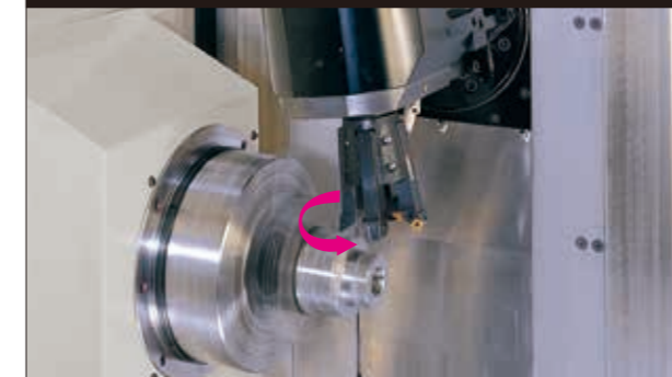
The tool can be indexed at fixed positions in 90 deg steps (4 positions) and tools can be used efficiently.
