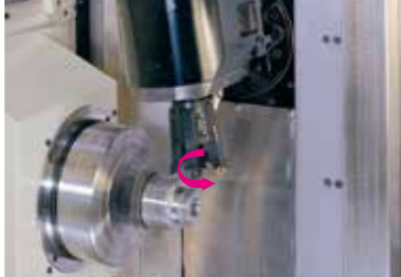
Multi turning holder to index in 4 positions
