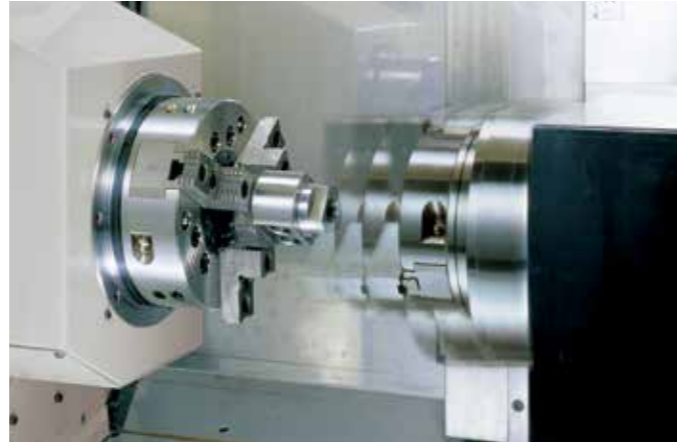
Multi turning holder to index in 4 positions
