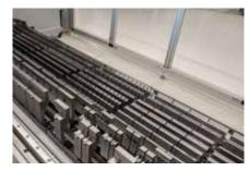
A stadium for two complete lengths of punches and five complete lengths of dies is integrated inside the machine.
