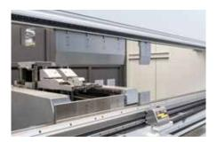
Quick-acting hydraulic clamping installed on the ram.
