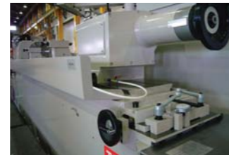
The photo is of a tailstock with 1,000kg specifications
