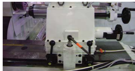
The photo is of a tailstock with 1,000kg specifications
