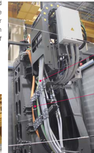
Wiring to Y-axis motor
