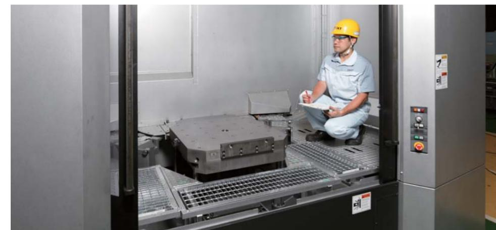
\* Execute pallet change after checking that the operator is out of the machine and the door is closed.
