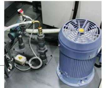
Spindle-through coolant 3MPa
